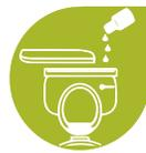
Put 15 drops of food colouring into the toilet cistern. If after 15 minutes the water in the toilet bowl has changed colour, there is a leak.
